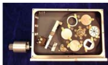
Internal Aperture Filter Wheel for InSb 1.0 \mu m-5.0 \mu m camera system
